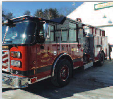
Holderness Fire Department — 12E3 Pierce Saber, 1000 Gallon tank, 1500 gpm Hale pump.
