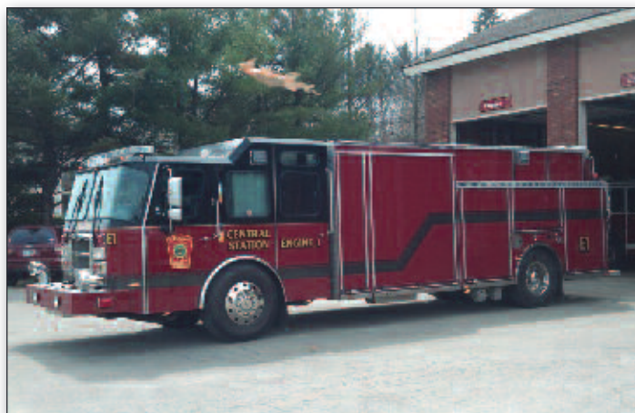
Laconia Fire Dept. — 13E1 2013 E-One 1,500 GPM pump, 1,000 gallon tank, class A foam tank, truck carries 1,600 feet of 4" capable of laying dual supply lines. Truck is equipped with 2 portable deck guns.
