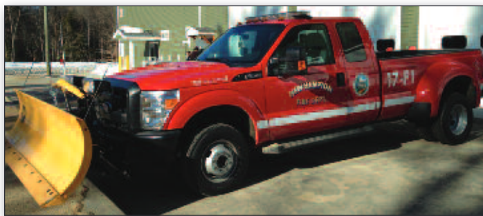
New Hampton Fire Department — 17F1 2014 Ford F350 4x4, dual wheels, 5-man cab. 9' plow. Skid unit with 350 gpm pump, 300 gal. water, 10 gal. foam with two electric hose reels. Towing capabilities, used as utility vehicle in off-season.
