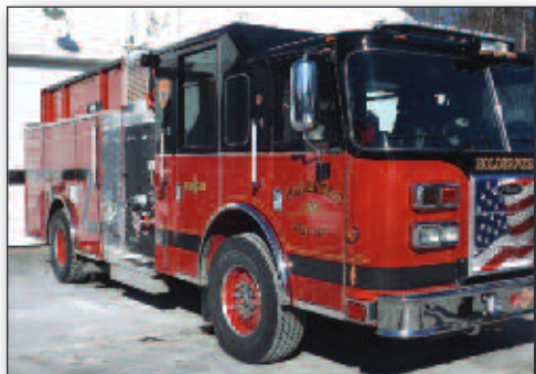
Holderness Fire Department — 12E3 Pierce Saber, 1000 Gallon tank, 1500 gpm Hale pump.
