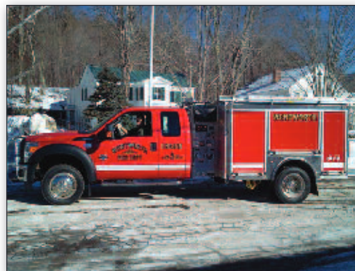
Wetworth Fire Department — 42E2 Engine 2 was designed as a quick attack piece, used for mva and various other calls. 500 gallon tank, 1,500 gpm pump, carries all extrication tools and rescue gear.
