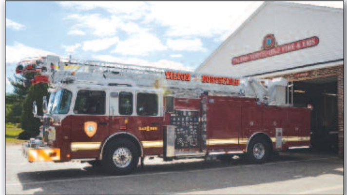
NEW APPARATUS Tilton-Northfield Fire Department. 21-Ladder-1 2013 Smeal. 75' Quint. 500 gallons. 55,000 lbs GVW. 6-person cab. 11'6" tall. 38' long.
