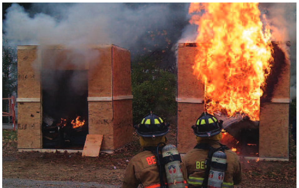
Below: The advantages of sprinklers become obvious in this demonstration created by the Belmont Fire Department at their October Open House.
