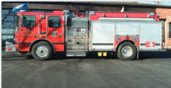
Center Harbor. 5E1 2011 HME. 1,650 g. water; 2,000 gpm pump; 1,600' of 4" hose; 9'8" ht; 29' long. 40,000 lbs. loaded with water and equipment. Heavy-duty axles.
