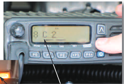
When an emergency signal is received at the Command Vehicle, a flashing yellow LED is activated and "EMG EMG" displays on the front of the radio, as well as the unit ID of the radio transmitting the signal.
