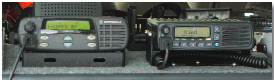
The radio on the left is monitoring the fireground channel while the radio on the right — the monitoring radio — is scanning all LRMA channels in case a "Mayday" is called on a channel other than the fireground channel.
