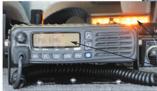
When an emergency signal is received at the Command Vehicle, a flashing yellow LED is activated and "EMG EMG" displays on the front of the radio, as well as the unit ID of the radio transmitting the signal.
