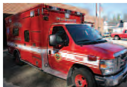
Plymouth. 18A2 2009 Road Rescue Ultra Medic on a Ford E-450 chassis. Custom cabinetry inside and out: roll-up door for access to Amkus power unit, increased interior stor- age includes a series of drawers. Also inside: med- ication refrigerator and IV warmers.
