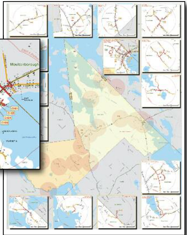
Above: Hydrant lines within the village area. Map at right shows overlapping circles where areas are served by hydrants.
